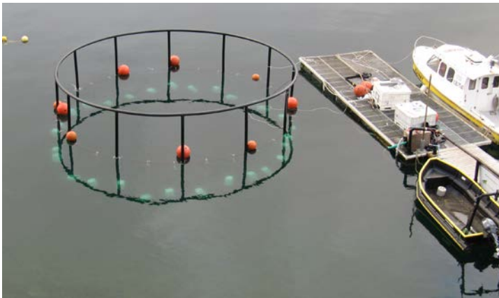
Figure 2: planned floating system for MESO-PAT in October/November 2014.
